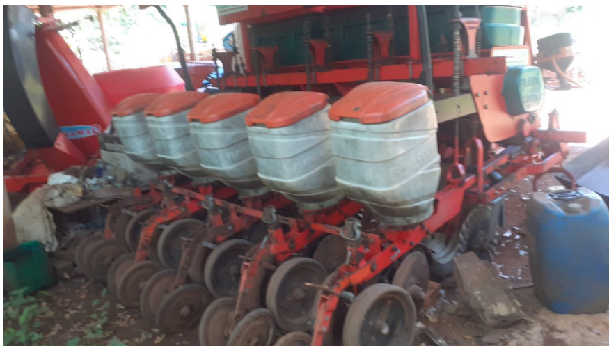
Figura 7 – Semeadora-adubadora 05 Planti-Center PC 5/3 2006. Coronel Freitas (SC), 2022
